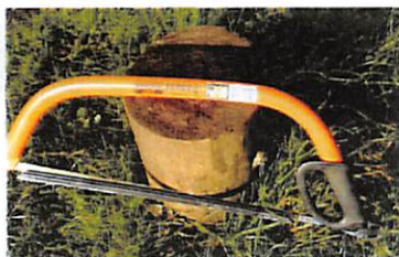
The bow saw has a guard to cover the blade. The guard must be put back on the blade after each use. The bow saws are to be put in a larger cupboard inside a container in the locked shed.
